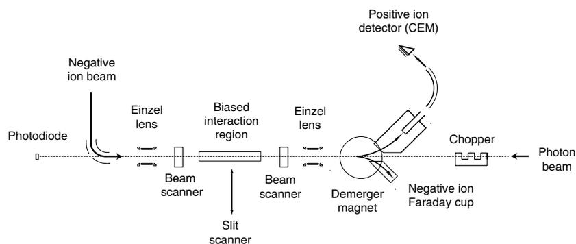
**Figure 2.** Schematic diagram of photon-negative ion merged beams apparatus
