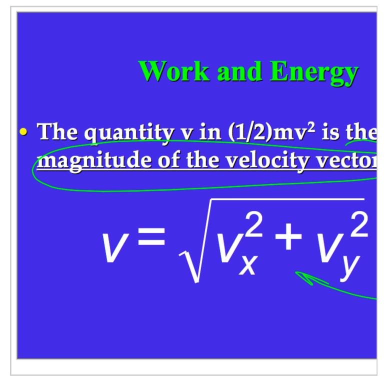
– Suppose a car has a mass of 1000 kg and is traveling at the rate of 20m/s, what is the kinetic energy of the car? What happens if its speed is tripled?halved? KE= Jmv2  $=\frac{1}{2}(1000 \text{ ks})(20 \text{ m})^{-1}$ = 200,000 J If v is tripled then KE increases by factor oz 9. IF v is halved, then KE decreases by factor
