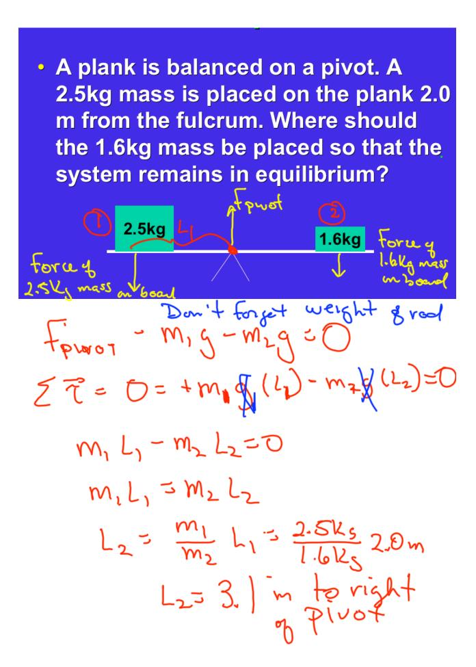
• A 2.0 kg plank is balanced on a pivot. The c.m. of plank is 0.50m to the right of the pivot point. A 2.5kg mass is placed on the plank 2.0 m from the fulcrum. Where should the 1.6kg mass be placed so that the system remains in equilibrium?
