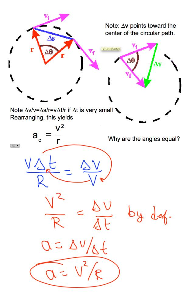
for uniform circular motion Vary = 5x = 17/ DX=2TTR At = time it takes to complete circle. This is called the period, T. Tis # sec per revolution f is # revolutions per second, this is called frequency  $V = \frac{2\pi R}{T} = 2\pi Rf$
