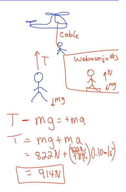
Now the man is accelerating in the upward direction at a rate of 1.10 m/s<sup>2</sup> and in the forward direction at a rate of 0.25 m/s<sup>2</sup>. What is the angle the cable makes with the vertical?
