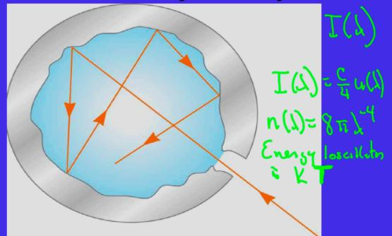
System is designed so that incident radiation has little chance of being reflected out before being absorbed by cavity walls. Goal calculate the energy density of EM waves in cavity.
