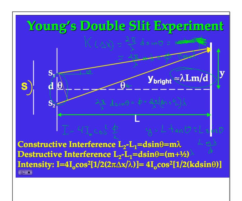
Red light from a He-Ne laser (λ=632.8nm) is incident on two narrow slits separated by 0.200mm. A fringe pattern is observed on a white sheet of paper held 1.00m away How far above and below the central axis do the first dark minima (minimum intensity) occur? Where is the 5th bright fringe.
