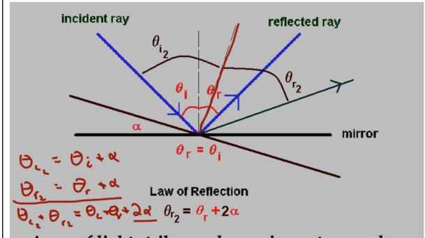
A ray of light strikes a plane mirror at an angle  $\theta$ . If the mirror is rotated by a, while the indent ray is kept fixed, the angle reflected ray rotates by  $2\alpha$ . Prove this.
