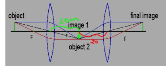
Can you derive an equation for the effective focal length of the lens combination? What is  $s_i$  if  $f_1$ =10cm,  $f_2$ =15cm, d=40cm, and  $s_o$ =20cm?
