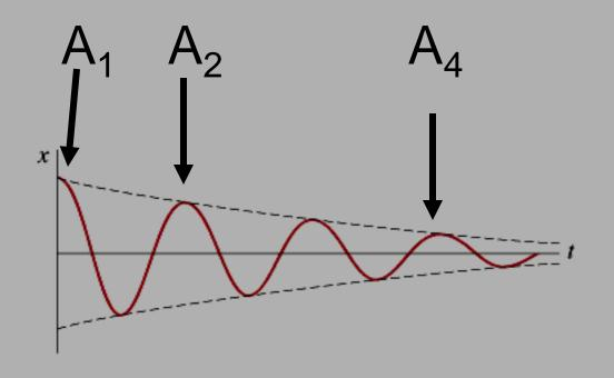
This is what happens when an oscillator is damped. This system is *underdamped*.
