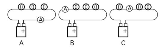
28. In which case is the current through the ammeter greatest?
