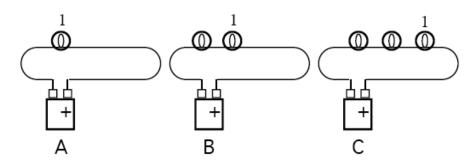
27. In which case is current through the ammeter greatest?
